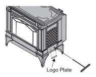
To adjust the aeration: use the allen key to turn the turning gear which will adjust the air shutter. Open the air shutter for a blue flame or close it for a more yellow flame. This adjustment is performed by a qualified installer. The factory setting should be sufficient for most installations.
